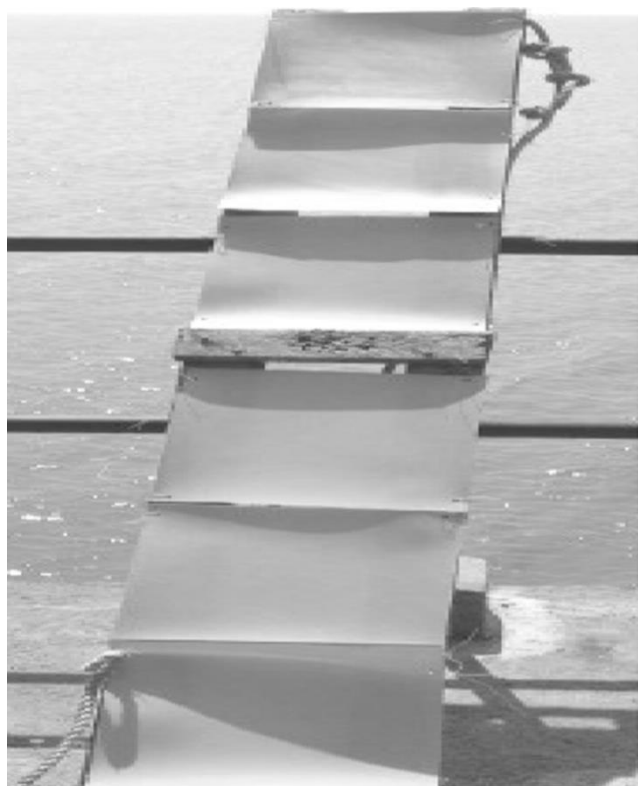
Figure 1. The Biofilm development rack.
